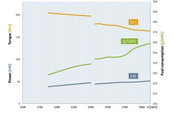
For the power ratings, refer to standard reference conditions of ISO 3046-1 (IFN): +25°C (77°F), 100 kPa, relative humidity 30%. The specified power is reached during the running-in period, and can be 5 % less on delivery. Power reduction acc. to ISO 3046-1. Standard values: More than 100 m above sea level approx. 1% per 100 m. Above 25 °C approx. 4% per 10 °C. The power taken from the alternator also has to be added to the power calculation.
