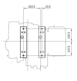
Spread at box dimensions  $\pm$  3 mm due to tolerance. Drawings with detail and connection dimensions as PDF resp. DXF can be found at www.hatz-diesel.com.
